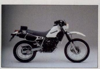
Kawasaki's KL250 offers a single-pot slice of Ninja know-how. Like the dual-purpose KL600, the 250 features two counterbalancers to combat vibration, single-shock Uni-Trak rear suspension, a removable aluminum sub-frame and a front disc brake. Claimed horsepower for the 250 is 28 bhp at the crank, and dry weight is 257 pounds.
