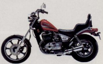
Filling the void left by the departed 550 LTD, the 454 parallel-Twin brings Ninja technology to the middleweight cruiser class. Sporting liquid-cooling, four valves per cylinder, a six-speed gearbox and belt drive, the 454 is claimed to produce nearly 50 hp and weigh under 400 pounds dry.
