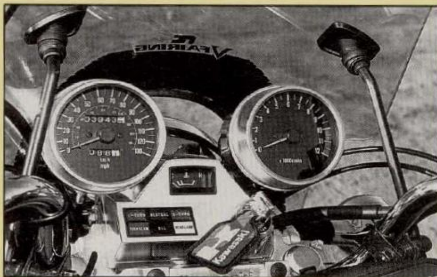
Instrumentation includes easy-to-read speedo and tach, engine temperature gauge, and turn/neutral/high-beam/oil lamps.
